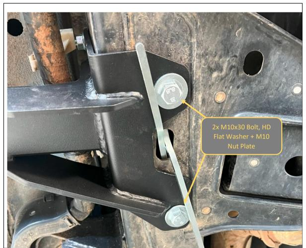
15. Once secure, finish front mount installation securing the lower mounting points with 2x M10x30 Bolts, HD flat washers and M10 Nut plates.
